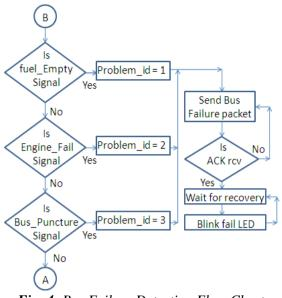
Fig. 4: Bus Failure Detection Flow Chart.
