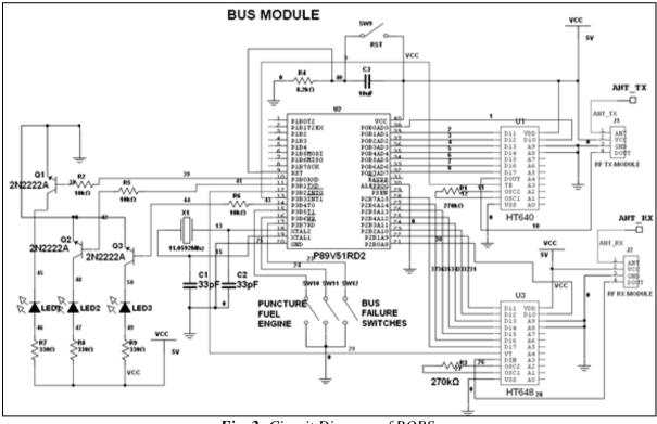
Fig. 2: Circuit Diagram of BOBS.
